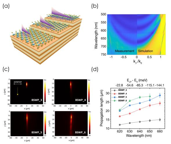
**Figure:** (a) Schematic of polariton systems comprising  $WS_2$  monolayers and distributed Bragg reflectors (DBR). (b) Measured and simulated angular reflectivity spectra of a polariton structure (BSWP-5). (c) Structure-dependent polariton propagation. (d) Comparison of wavelength-dependent propagation lengths for different samples.
