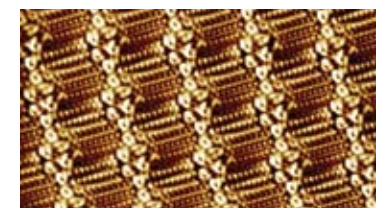
STM image of a nanopatterned surface decorated with clusters of aromatic rings spaced by alkane chains
