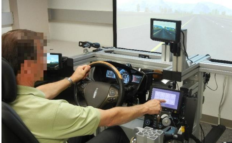
Figure 1. A button search-and-press task on a touch screen in a fix-based driving simulator
