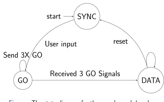
Figure: The state diagram for the encoder and decoder.
