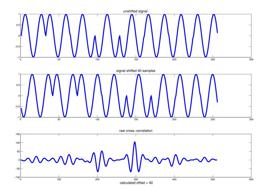
Figure: An example of a signal cross-correlated with a shifted version of itself. The maximum value of the cross-correlation shows how big the shift is.
